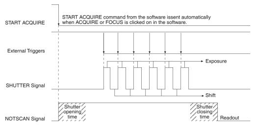
Figure 24. Multiple Trigger Timing Diagram
